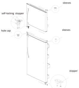
9.Put down the refrigerator door bottom hinge vertically, take out the the middle hinge of the other side from the accessory bag then assemble the middle hinge on.
