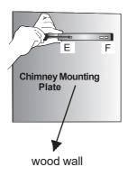
Screw the chimney mounting parts into Ø 8mm sized wall plugs on E,F points which is provided with your product.
